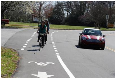
Bike lanes provide a striped travel lane on roadways for bicyclists.
