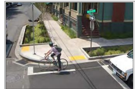
Bicycle forward stop bars encourage cyclists to wait where they are more visible.
