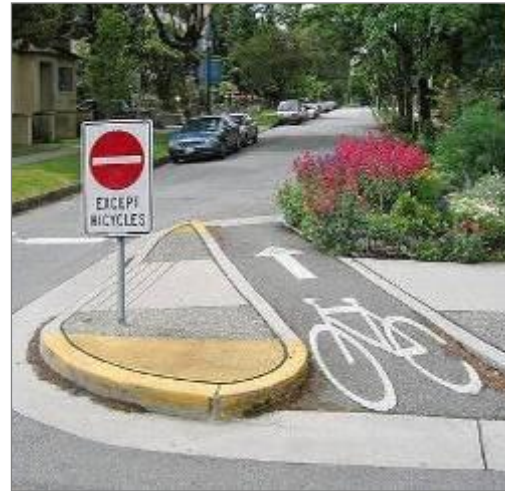
Choker entrances prevent vehicular traffic from turning from a main street onto a traffic-calmed bicycle boulevard.
