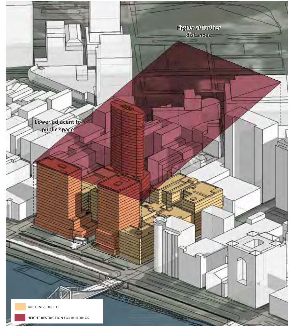
An inclined plane restricting height preserves views of public spaces and prevents overshadowing
