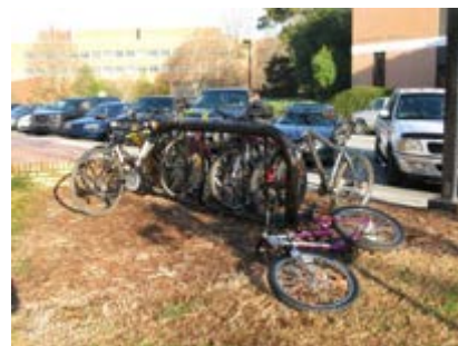
Bike rack over capacity. Design prohibits proper bike frame support. Near Lowry Hall.
