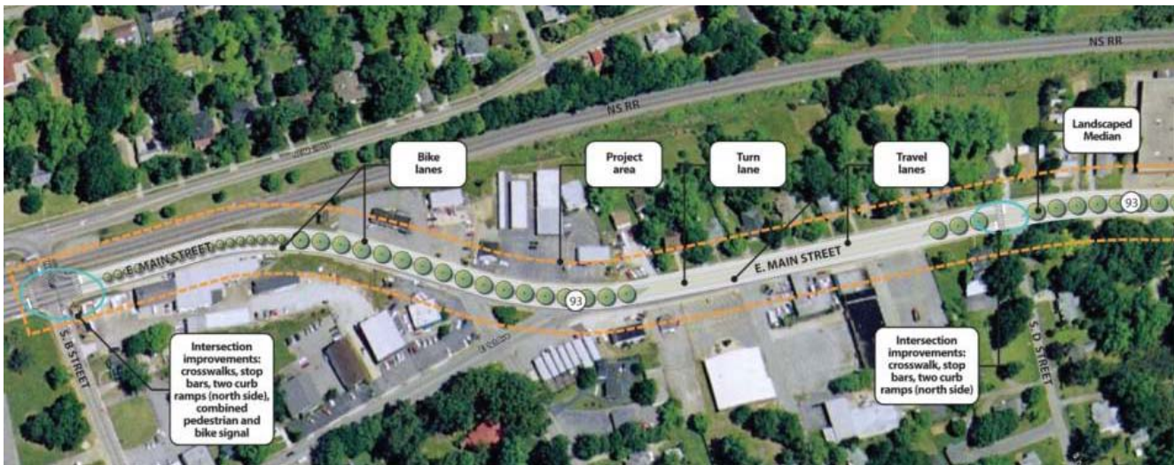
Intersection improvements at S B St and S D St, bike lanes along corridor, landscaped median in places
