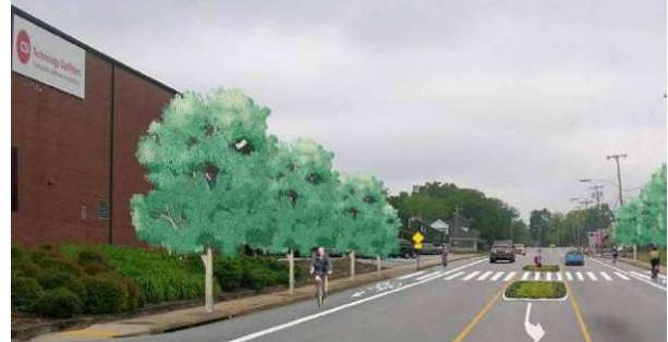
Reduce to two-lane street, add bike lanes, high-visibility crossings with islands, and a median
