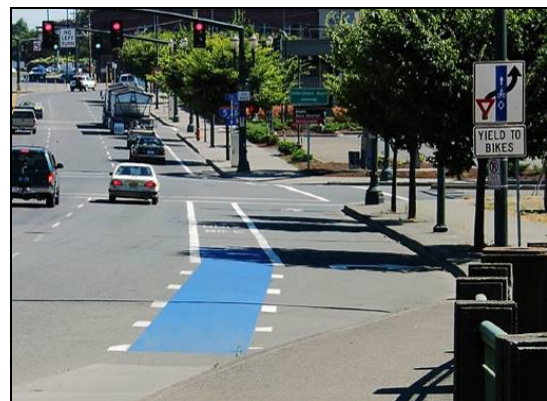
Portland, OR implemented blue bike lanes and has since changed to green
