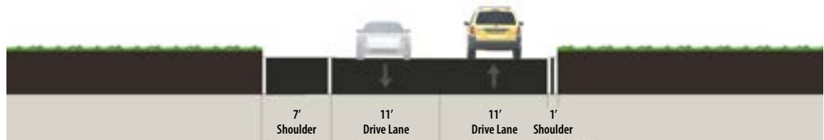
East Bramlett Road Bridge Segment - Proposed Design Changes (Option 1): Reduce vehicle lane size on the bridge segment (over the railroad adjacent to the Swamp Rabbit Trail) from 12 feet to 11 feet to allow a wider shoulder on the south side for pedestrians and cyclists, which would connect to the new sidewalk.
