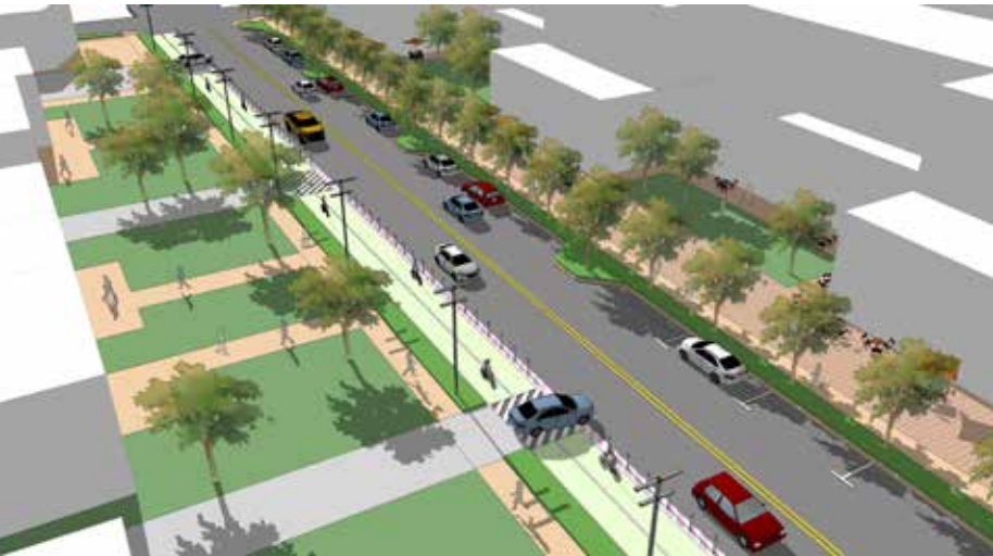
Pendleton Street Alternative A — This option includes a two-way buffered cycle track and new sidewalks on one side and on-street parking with expanded pedestrian zone on the other side
