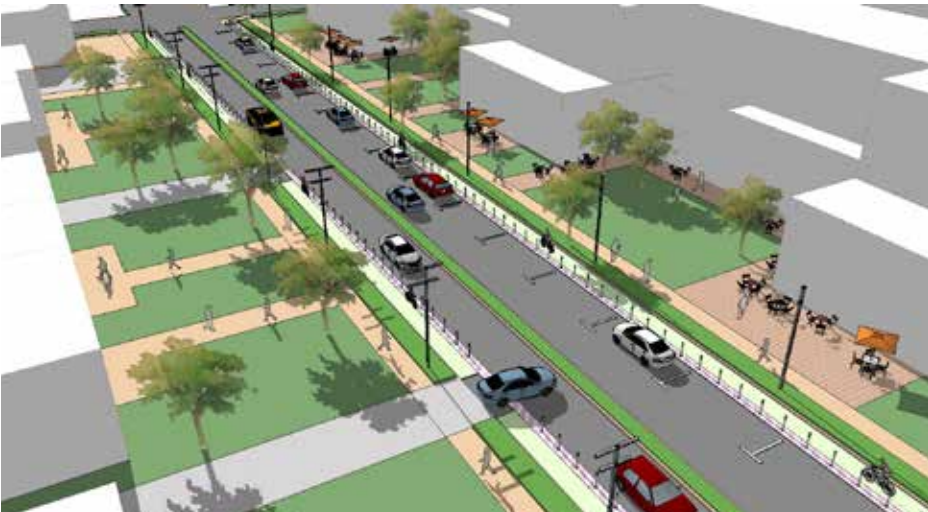
Pendleton Street Alternative C — this option illustrates protected bicycle lanes on both sides of the street with on-street parking on one side
