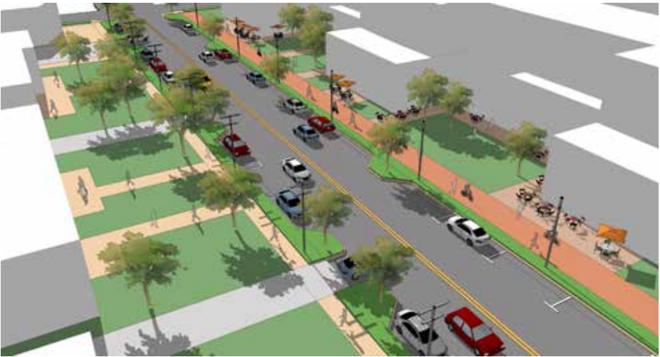
Pendleton Street Alternative B — This option features a Multi-use path along one side with on-street parking on both sides *Community feedback indicated a preference for separate bike and pedestrian infrastructure
