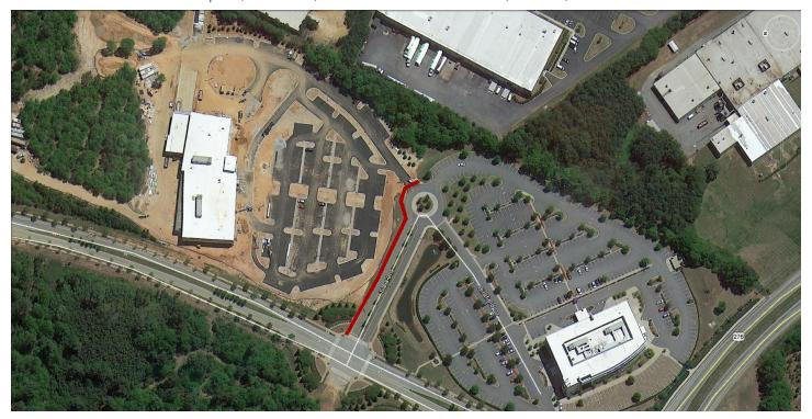
The existing sidewalks connecting to Innovation Drive will need to be widened to 10' to allow for multi-modal use. Additional pedestrian crossing improvements will be required along Sara Lane at the existing internal roundabout.
