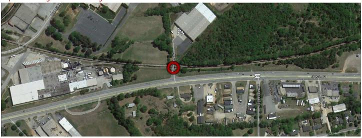
An existing vehicular rail line crossing at the entrance to the Heafner Tire gives an alternative to the pedestrian only crossing at the existing ROW, as shown above. This crossing will need to be improved for bicycle and pedestrian use, and approved by Carolina Piedmont Rail. The graphic below shows a typical railway crossing for a multi-use trail allowing for safe bicycle/pedestrian crossings (AASHTO 2012: *Guide for the Development of Bicycle Facilities*).
